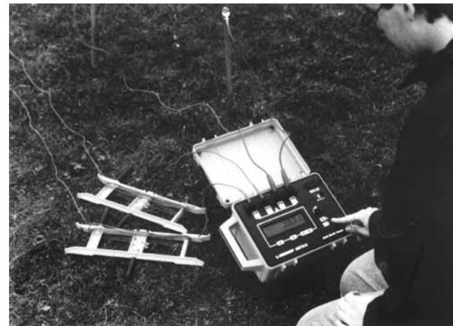
The Megger DET2/2 ground tester offers additional features for testing in a high-noise environment
