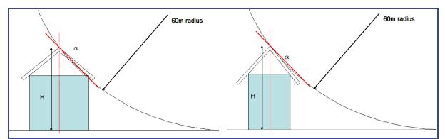
The area under the zone of protection is the same with or without the eave, with respect to the rolling sphere we can see in the above example how it may also offer protection to the eaves. The above example also shows a shallower pitch where eaves protection would be needed.
