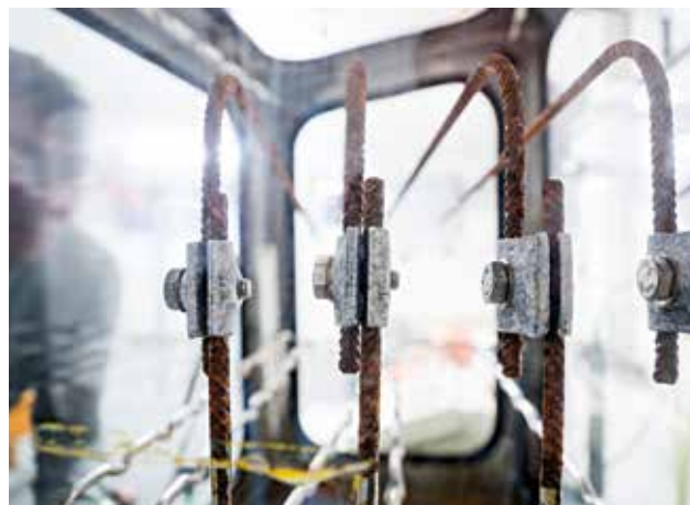
Figure 1.26: BET SO 2 testing system
