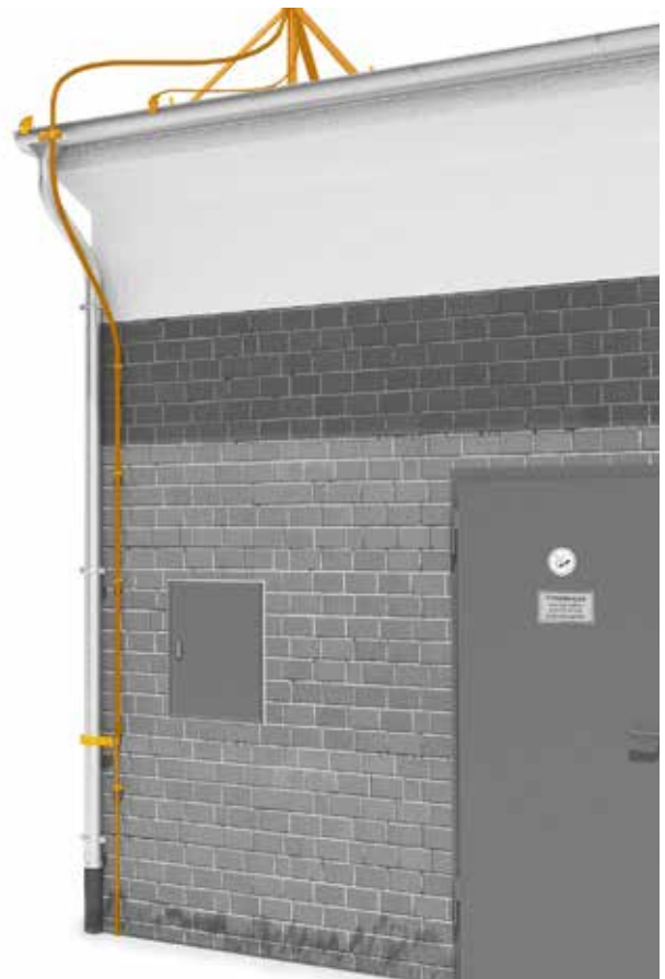
Figure 2.56: Example: protection of a gas distribution point with isCon® cable
