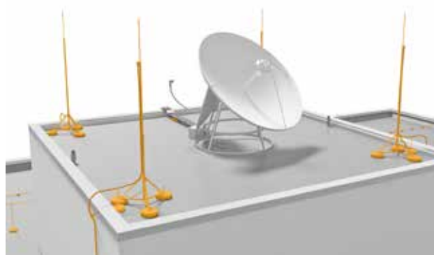
Figure 2.61: Isolated lightning protection with interception rods
