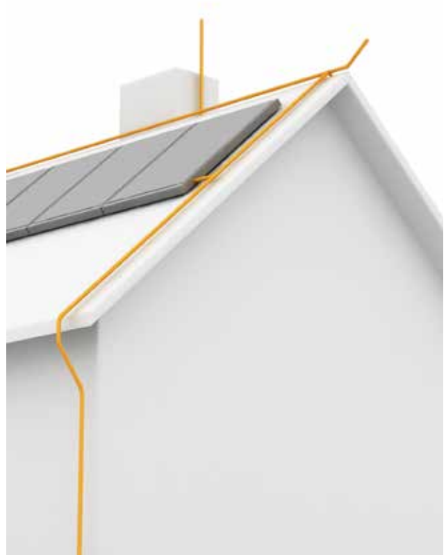
Figure 2.19: Direct connection of PV mounting frames to the lightning protection down-conductor system
