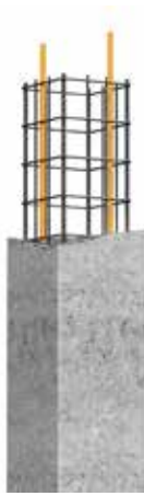
Figure 2.53: Example: use of reinforced concrete supports/down-conductor system
