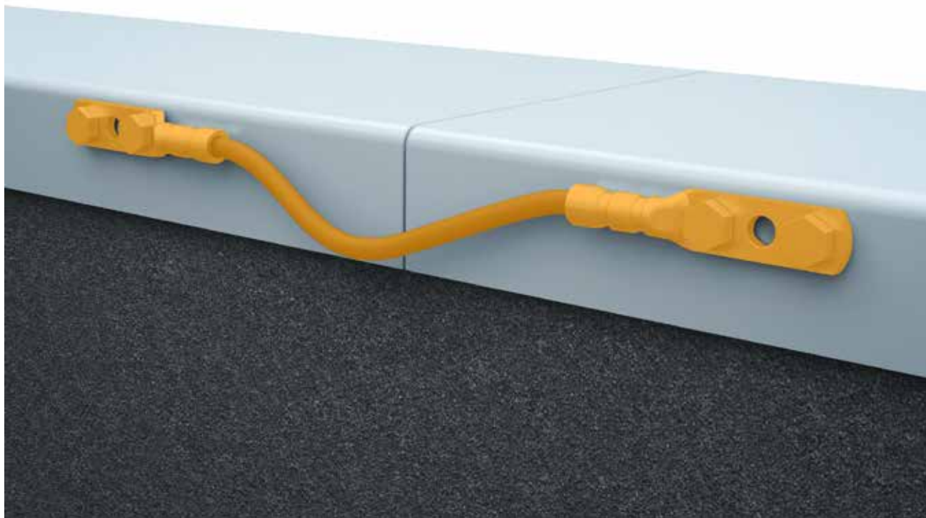
Figure 2.15: Possible method for connecting metal on roof parapet by bridging with a flexible cable
