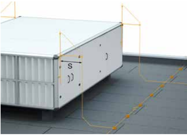
Figure 2.32: Example: air-termination system with Iso-combination set for triangular fastening
