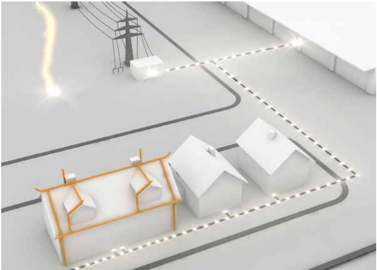
Fig. 1.14: Danger: galvanically coupled and line-carried surge voltage
