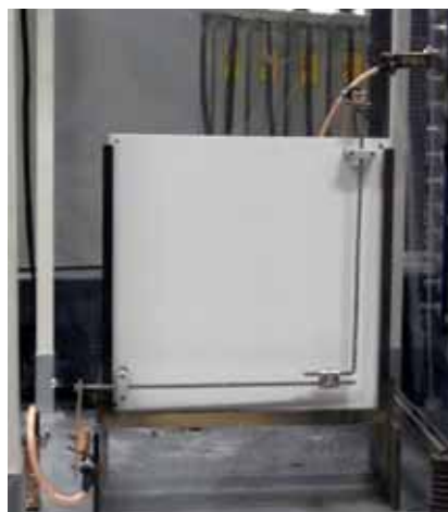
Figure 5: Specimen fixed on insulating plate (MV clamp) for a test in the impulse current laboratory.
