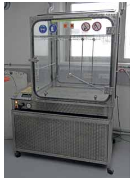
Figure 2: Test in a Kesternich chamber.
