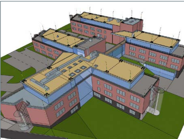
Positioning of the air-termination systems
