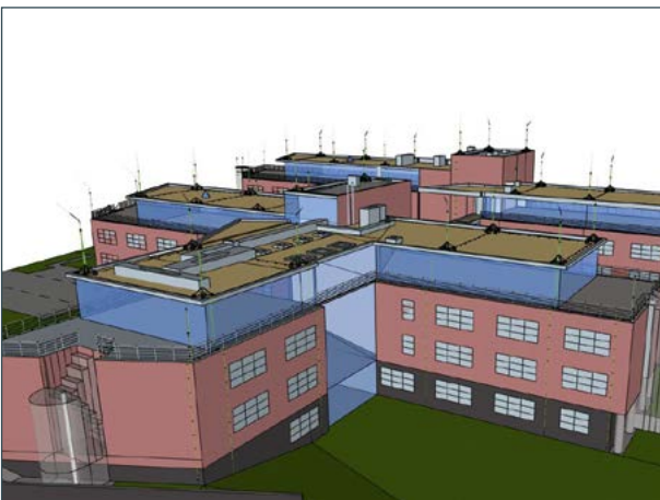
Positioning of the air-termination systems
