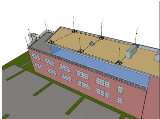
Positioning of the air-termination systems
