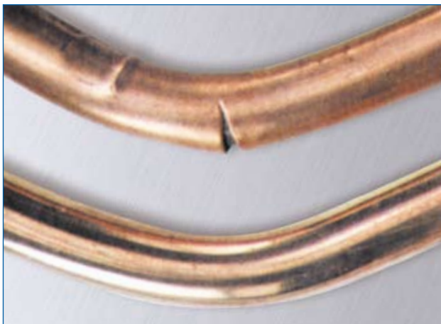
Figure 76. Copper bonded and copper clad earth rods.
