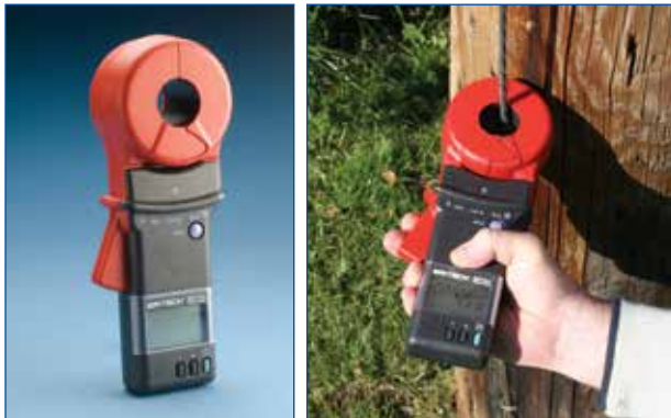
Figure 74. Pentair test equipment for resistance and resistivity measurements.
