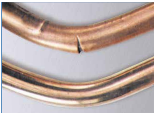
Figure 76. Copper bonded and copper clad earth rods.
